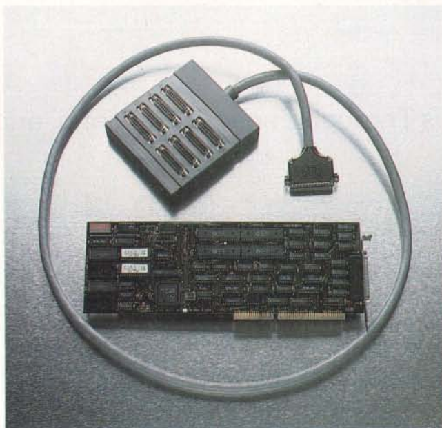
The IntelliPort AT8 is an eight-port I/O board.
