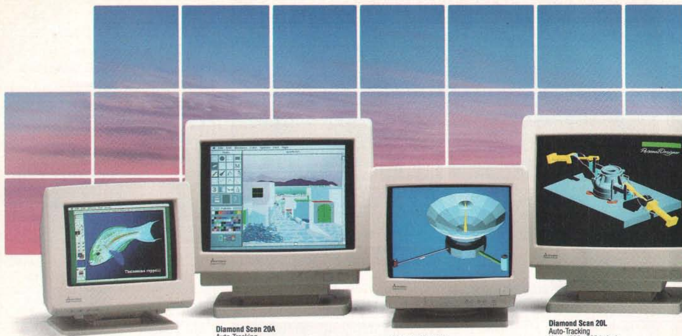
Diamond Scan 14 Auto-Tracking 800 x 600 pixels (digital, analog, monochrome) 330 x 500 pixels (composite NTSC)
