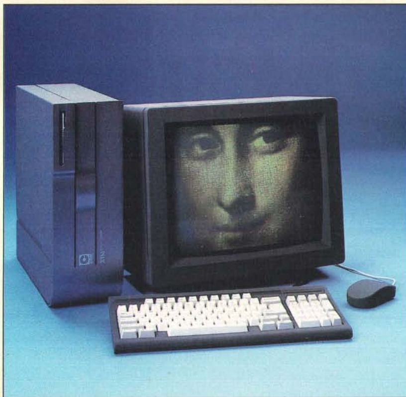
Photo A: Cogent Research's XTM parallel desktop supercomputer, based on the INMOS T800 transputer and Yale University's Linda programming language. (Photo courtesy of Cogent Research, Inc.)
