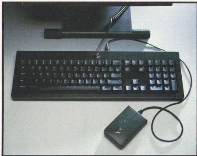
Photo 3: The cube's keyboard. The keys above the cursor keys control the monitor's brightness, the system's power, and sound volume.
